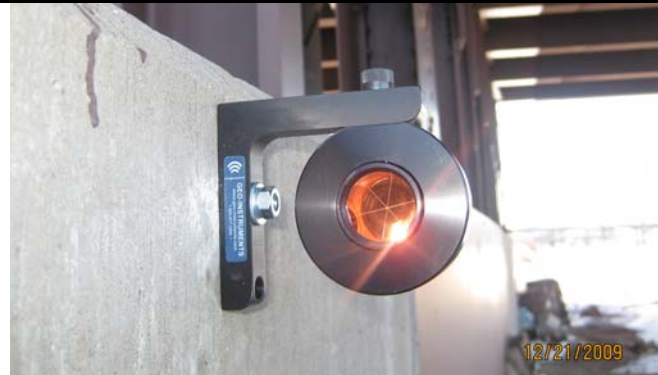
Prism on Abutment of 43 rd Street Bridge.
