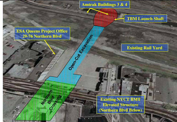
Queens Open-Cut Excavation (Northern Blvd to Existing Rail Yard).
