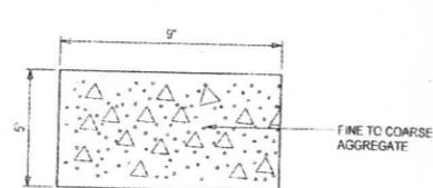
CORE WAS RETRIEVED IN ONE PIECE CORE CONSISTS OF FINE TO COARSE AGGREGATE IN A GRAYISH MATRIX. CORE HAS NOTICEABLE AIR CAVITIES AND PINHOLES.
