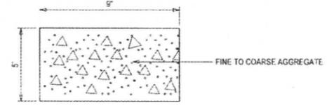
CORE WAS RETRIEVED IN ONE PIECE CORE CONSISTS OF FINE TO COARSE AGGREGATE IN A GRAYISH MATRIX CORE HAS NOTICEABLE AIR CAVITIES AND PINHOLES.
