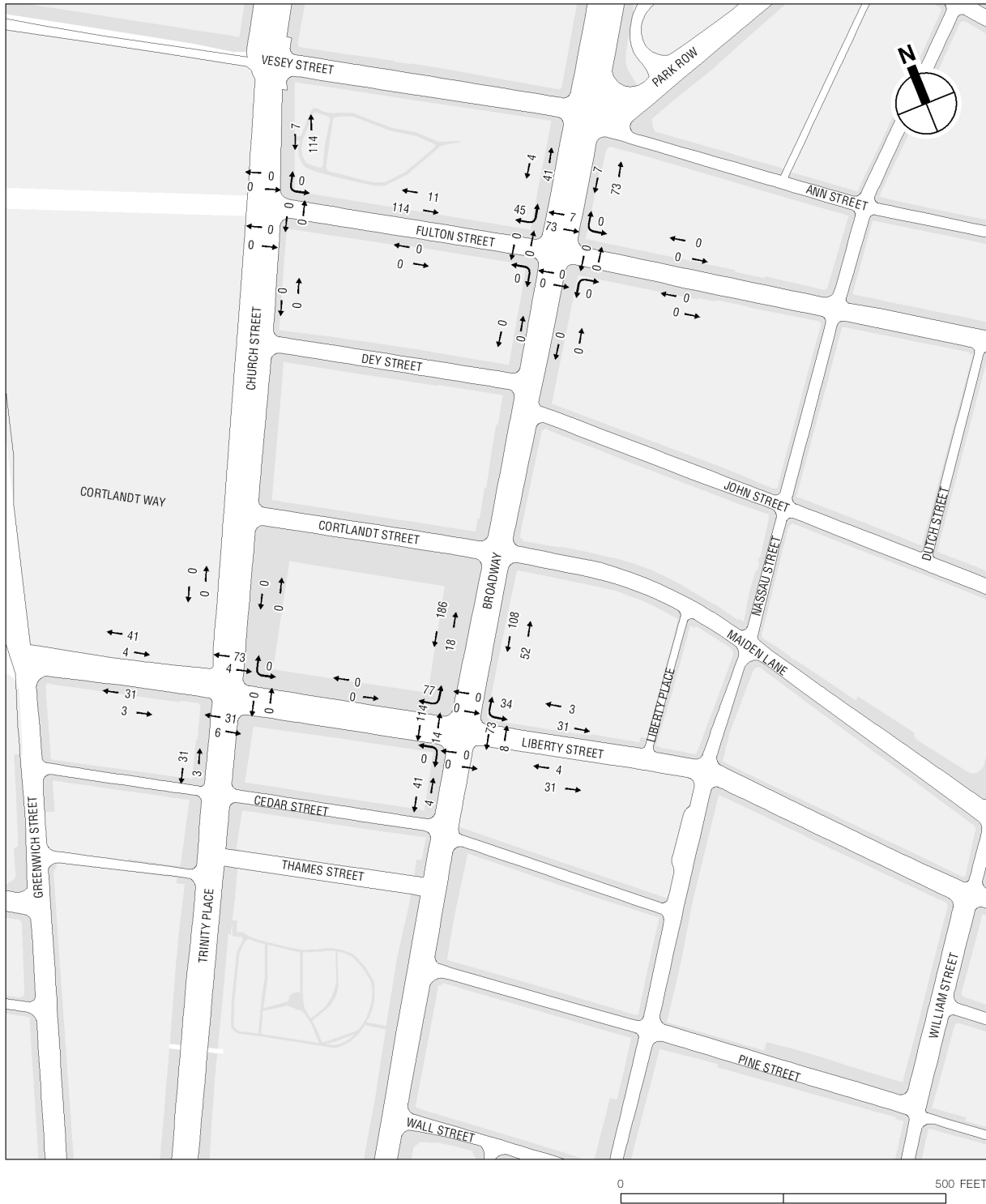
Figure 4E.3-11. Project Generated Pedestrian Trips – World Trade Center/Fulton Street Study Area: Weekday AM Peak Hour
