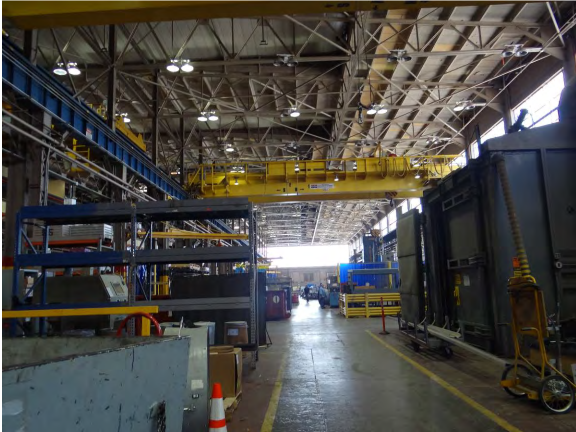
Photo 15. Former NYNH&H Railroad Van Nest Electric Locomotive Repair Shops. 60 Ton Overhead Crane, 2013.
