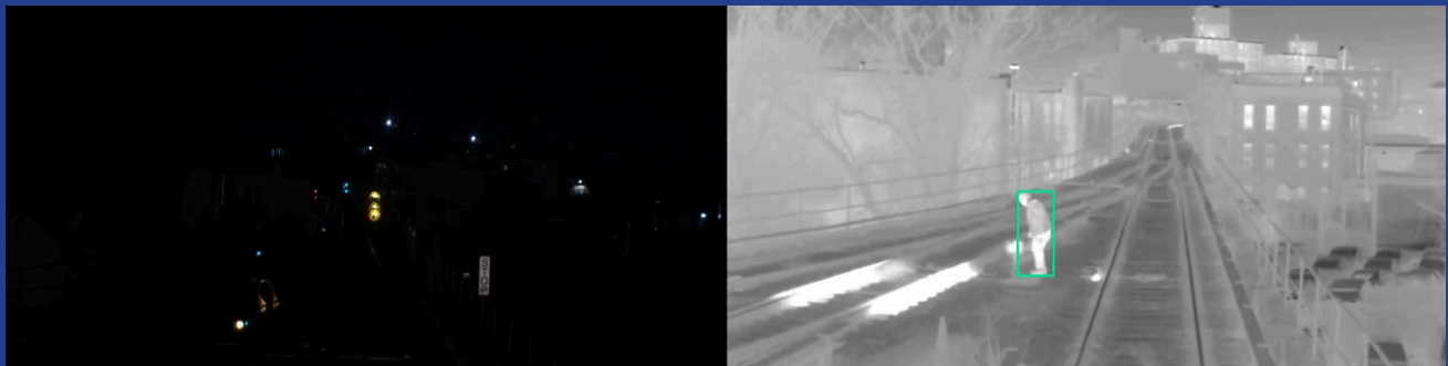
Front-facing cameras on trains can detect individuals and objects on the tracks even in low-light conditions.
