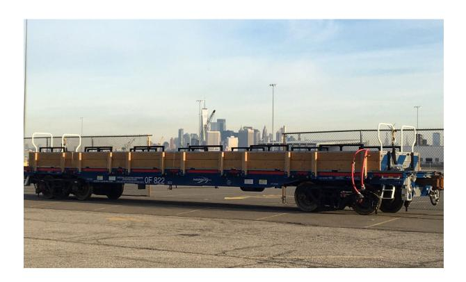
Pictured above is an R252 flatcar. This month's Committee agenda contains the exercise of an option to purchase an additional 52 flatcars, as well as related non-car items such as spare parts and technical documentation. When moved by a locomotive, flatcars are used throughout the system to transport track maintenance machinery and other heavy equipment, materials, and supplies used to support work at various NYC Transit locations.
