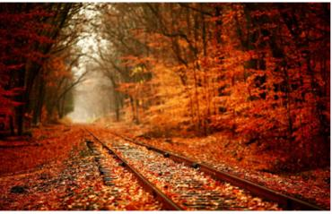
slow down during your commute, the gelatinous "slime" created by dead autumn leaves can result in a condition known as "slip slide" — causing the wheels to slip or slide along the rails.
