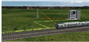
where all Metro-North trains automatically communicate in real-time with wayside locations and our Operations Control Center regarding train position, speed and actions of our locomotive engineers. For example, if a train is traveling too fast, the safety system will automatically take control of the train, bring it down to a safe operating speed and
