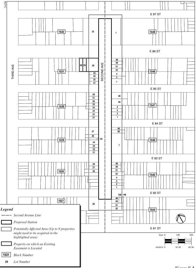
Figure F-5 86th Street Station Study Area for Potential Easements or Acquisitions
