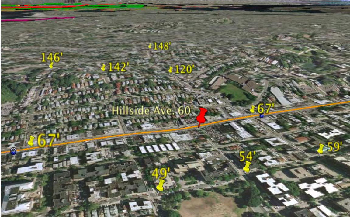
Figure 12: Hillside Avenue, Queens, with F-subway (orange-brown line) and elevations (ft) for selected points. The NYCT Pump Station is below the red pin, where Hillside Ave. and the F line tracks (which are 30 ft below grade) are the lowest. Run-off from the terminal moraine hills to the north contributes to the flooding. See text for details.
