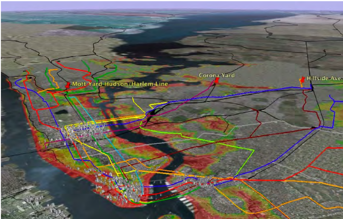
Figure 1: Location of the 3 case study sites: NYCT Hillside Ave. Pump Station on the F-line Metro-North; NYCT / LIRR Corona/Shea Yards – Flushing Meadows, Queens; and Mott Yard (Bronx). Colored areas are worst-track storm surge flood zones for Saffir -Simpson Category-1 in red, SS2 in yellow, SS3 in brown, and SS4 in green. Colored lines are subways, black lines are rail systems. See text for details.
