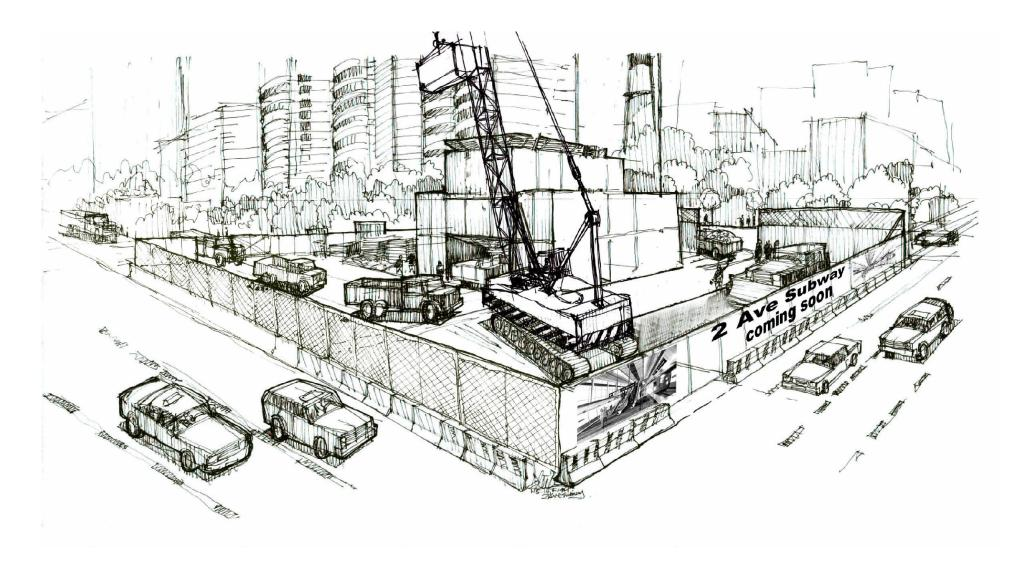
Figure 12-4 Conceptual Illustration of 12'-High Noise Barrier Encircling Playground 96 and/or St. Vartan Park
