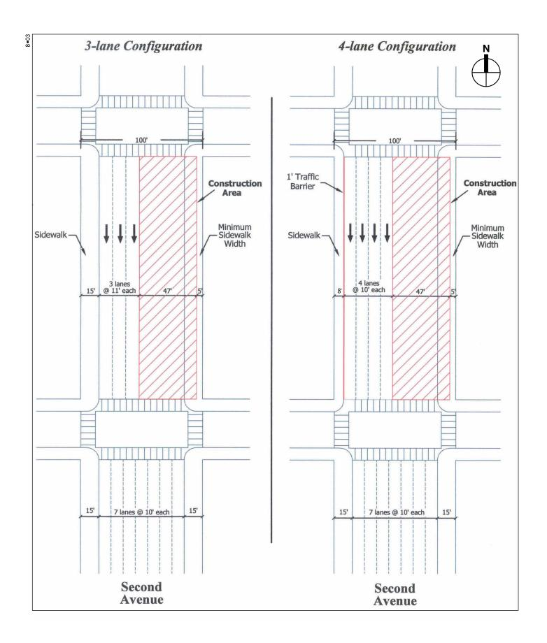
Figure 5D-2 Roadway Configuration Options During the Decking Installation Construction Phase
