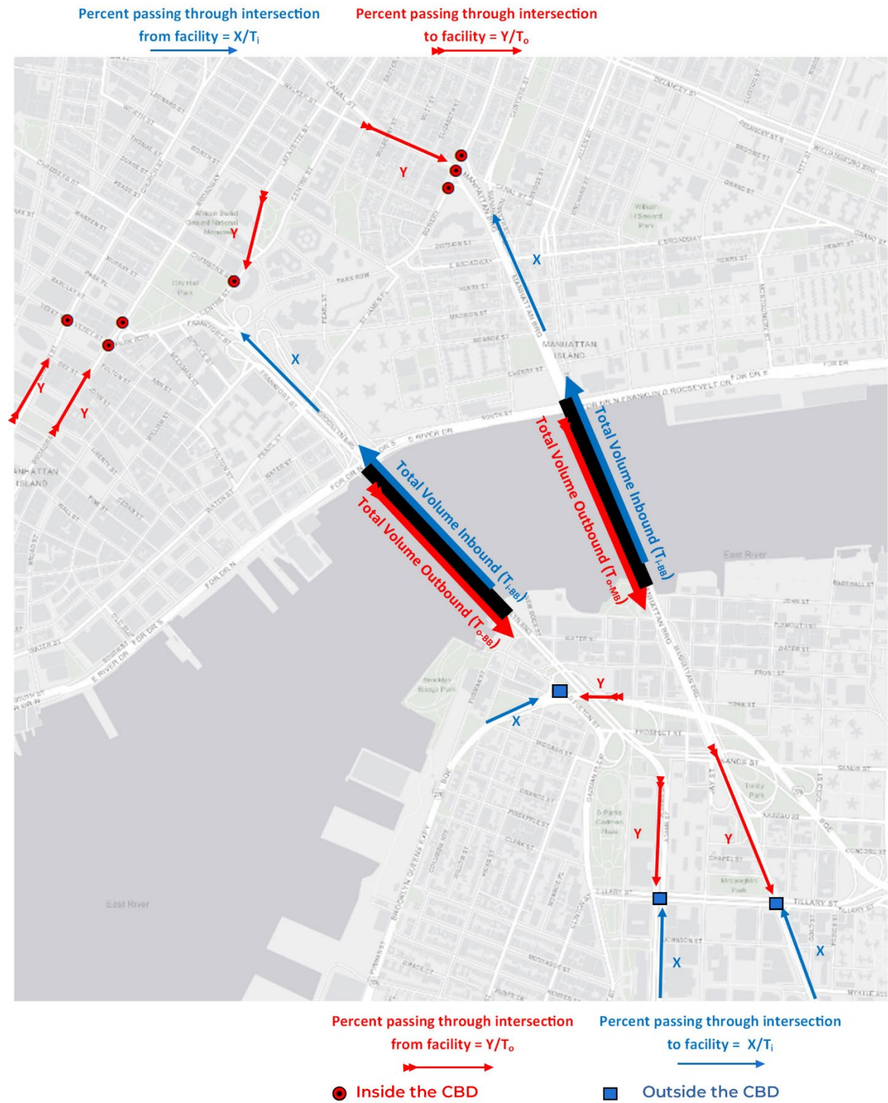
Figure A-3 Traffic Assignment to Specific Intersections
