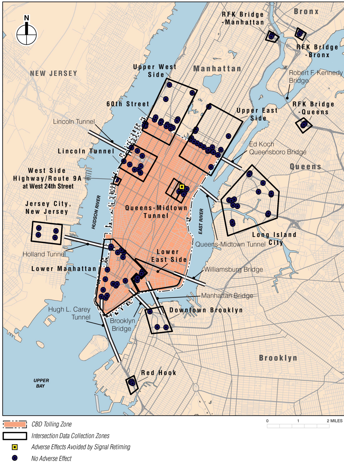
Figure 4B-17. Potential Adverse Traffic Effects at Local Intersections Late Night (LN) Period
