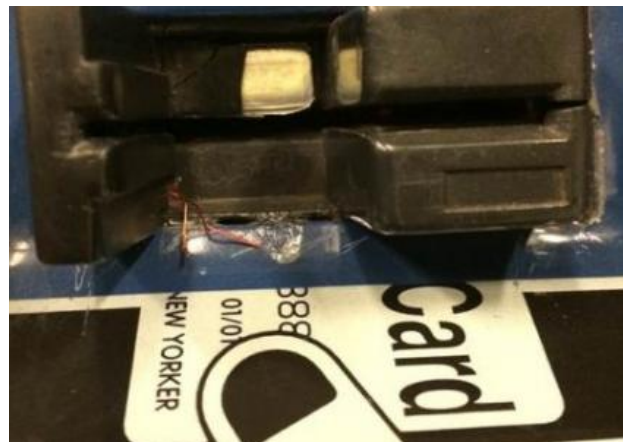
Wires and battery of skimming device
