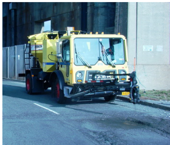
MTA Bridges and Tunnels' RoadPatcher truck, which can fill as many as 100 potholes in a single shift, working at the Robert F. Kennedy Bridge.
