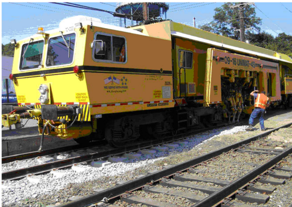
High production Unimat Tamper – lifts and aligns track
