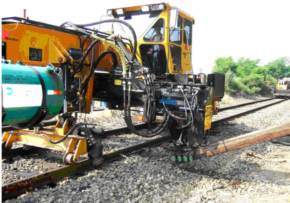
Tripp Machine – Purchased in 2005 removes and installs ties
