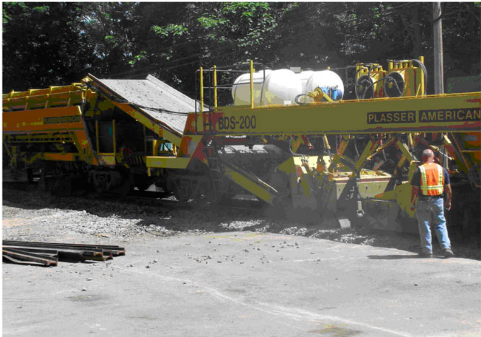
Ballast Distribution System – picks up excess stone
