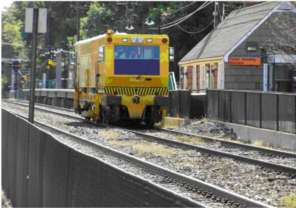
Stabilizer locks in stone ballast with vibration
