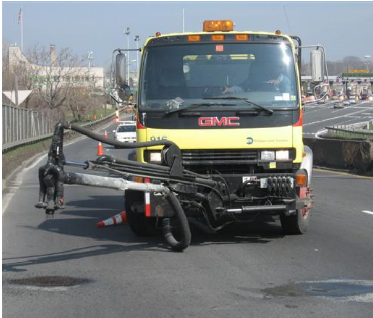
MTA Bridges and Tunnels' odd-looking but efficient Roadpatcher machine hard at work on the Bronx-Whitestone Bridge.
