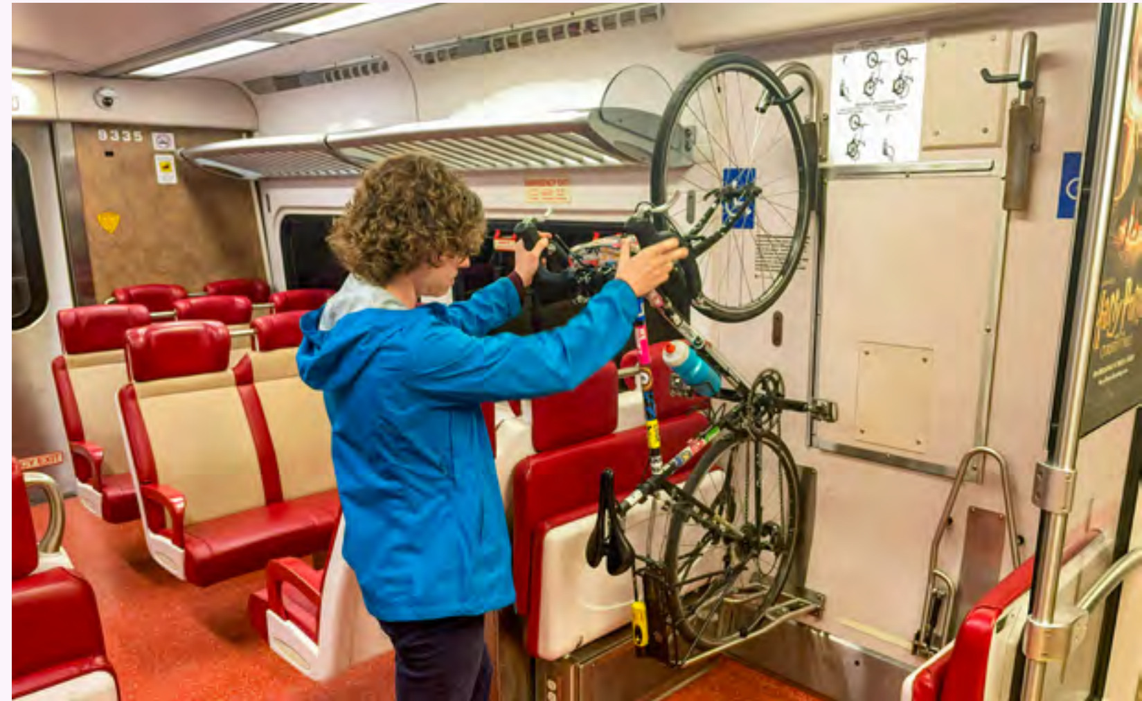
Wall-mounted bike racks on Metro-North Railroad New Haven Line train. (Source: Emily Provonsha/MTA.)
